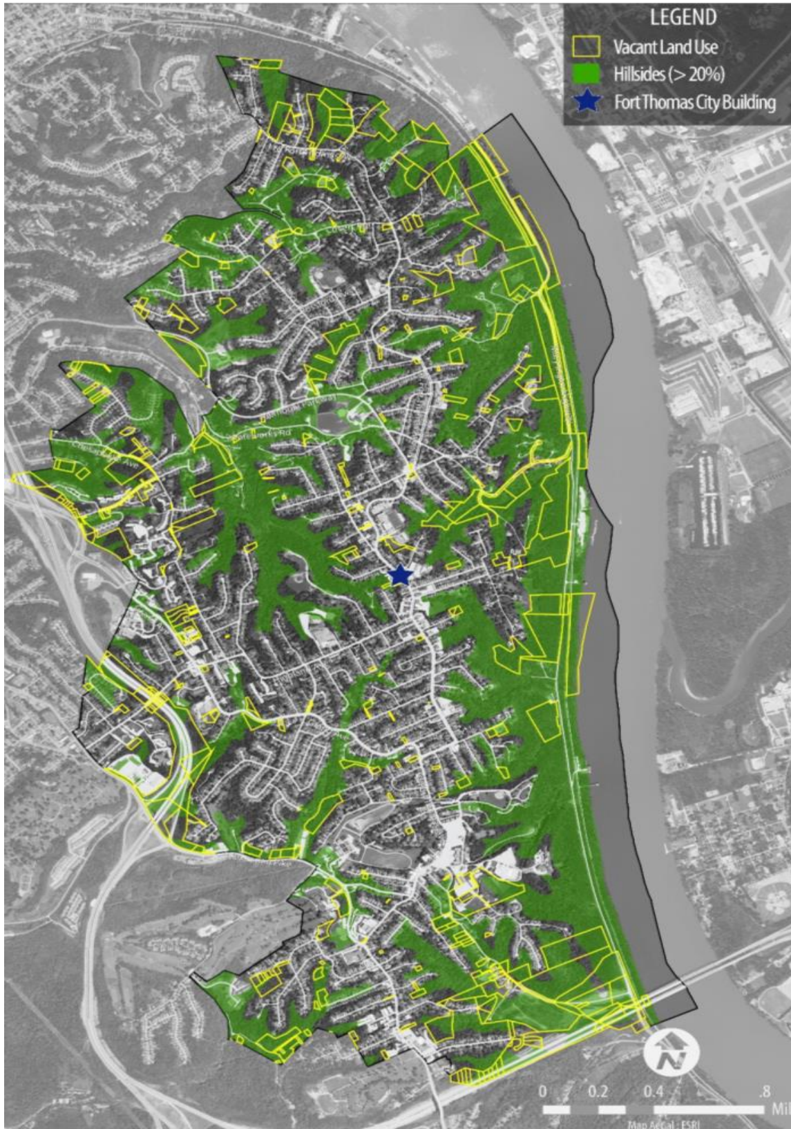
Figure 5.2-1 - Slopes Greater than 20%
