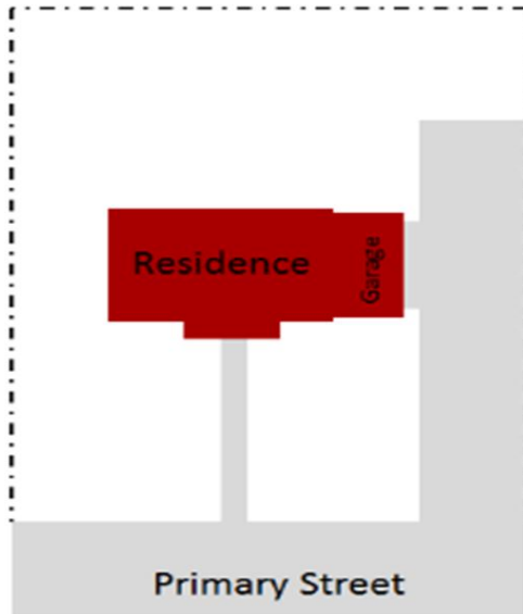
Figure 3.8-3 - Illustration of an attached side-loaded garage that is recessed from the front facade of the dwelling
